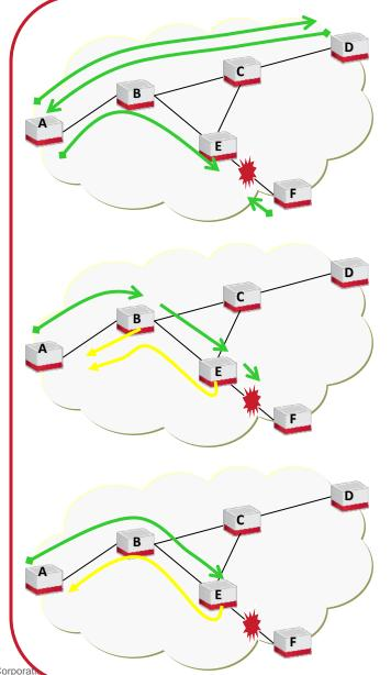
Continuity check messages (CCMs) dispatched over service to detect continuity and connectivity faults within service connection
