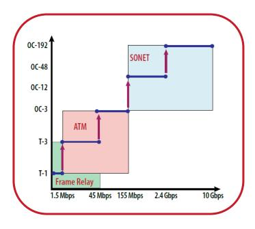
Carrier/Metro Ethernet addresses the limitations of legacy technology by providing flexible bandwidth scalability
